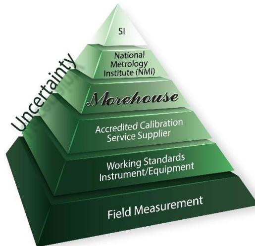
Figure 2: Metrological Traceability Pyramid for Force Measurement
