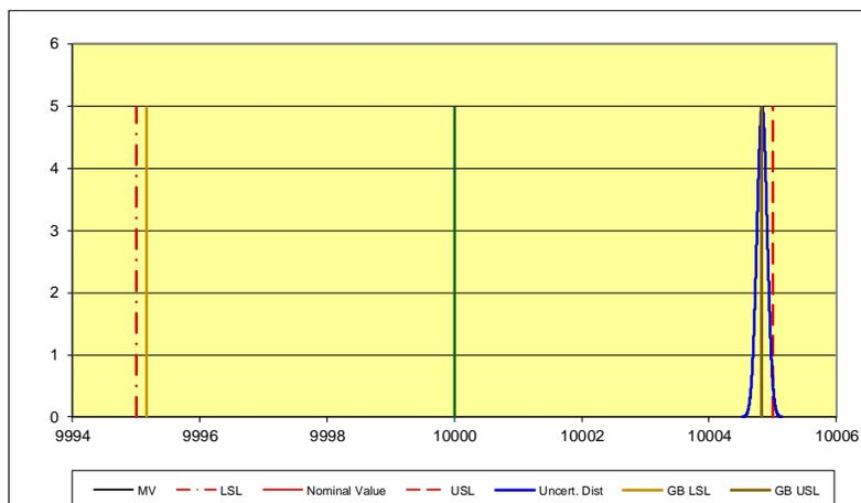
Figure 2: Guard band USL showing a 2 % PFA when Measured Value is at the GB USL
