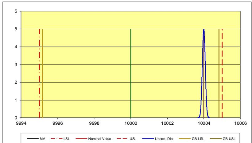
Figure 3: Graph Showing 10,004 as the measured value with a 31.23:1 TUR which is achieved by using a lab with low uncertainties
