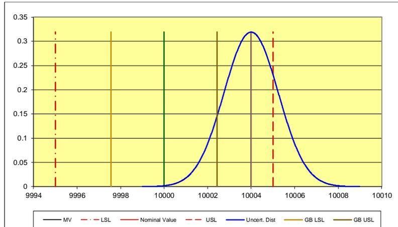
Figure 4: Graph Showing 10,004 as the measured value with a 1.99:1 TUR as the labs Expanded Uncertainty is higher than in figure 4
