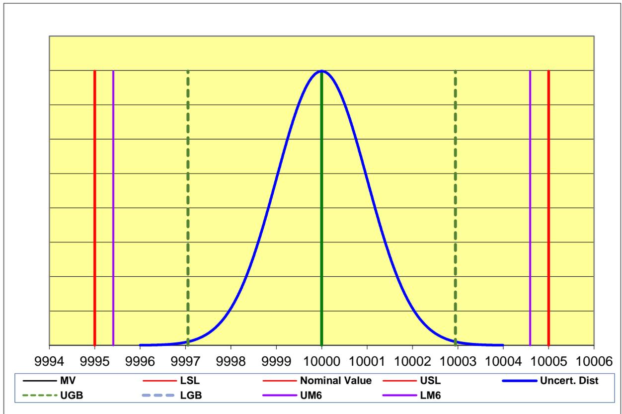
Figure 5: Graph Showing Specification Limits and Acceptance Limits for Both Method 5 and Method 6
